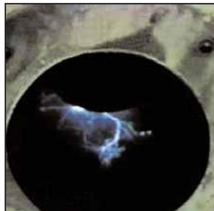
Figure 2. Spark Discharge within Oil Reservoir
