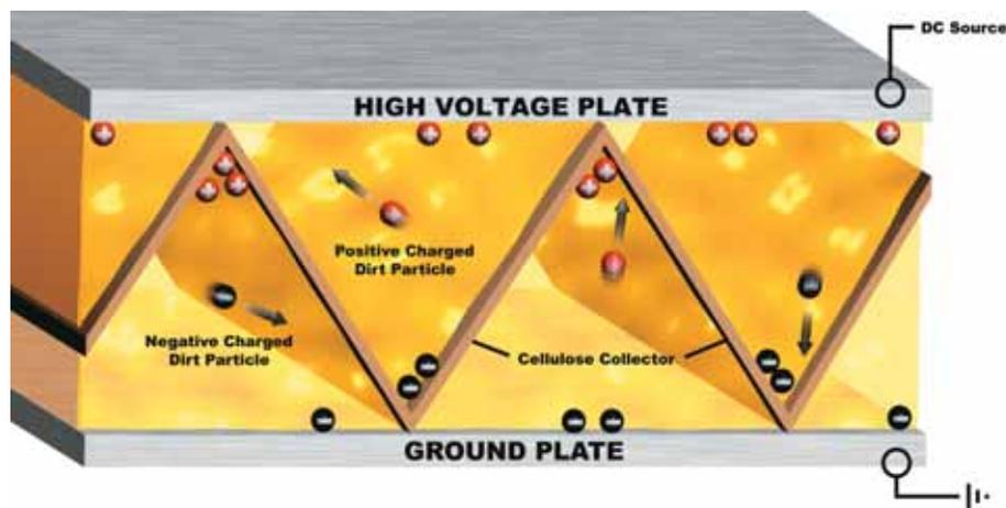
Figure 4. Electrostatic Collection
