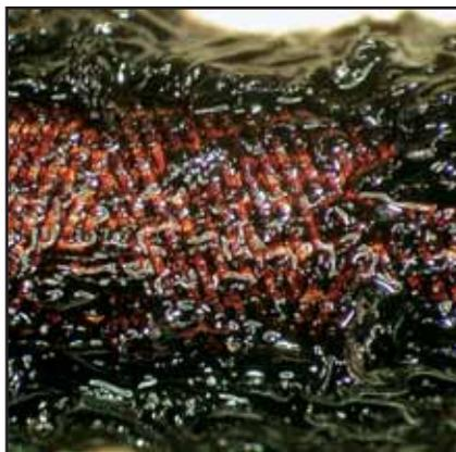
Figure 1b. Varnished Pencil Filter
