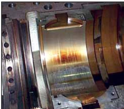
Figure 1a. Varnish on Shaft
