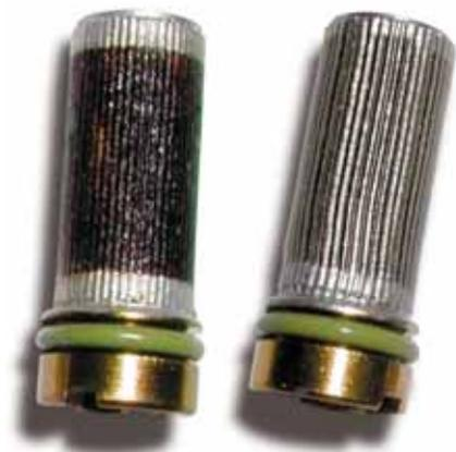
Figure 5. Varnished Servovalve Before and After 45 Days of Electrostatic Cleaning
