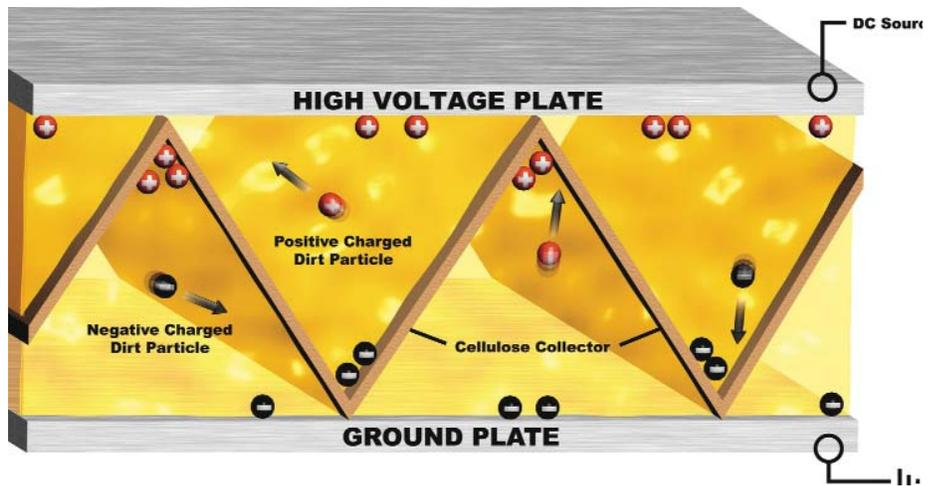
Figure 1: Cellulose collectors in the electrostatic cleaning system replace mechanical filters
