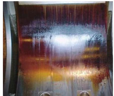
Figure 2: Varnish can accelerate the wear of components and cause valve stiction
